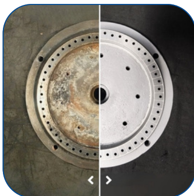
Refurbishing van Die Plates
